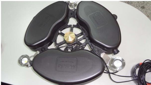
4, Arranging the LED and pump cables
