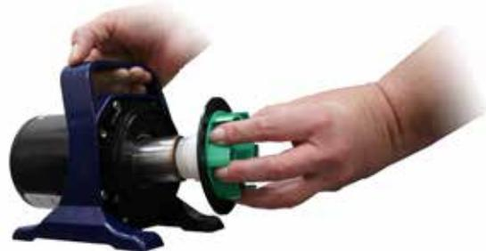
**5** If your impeller and internal pump body have excessive scale build-up, clean with a mild acid, such as white vinegar or non-abrasive calcium, lime and rust remover product using a sponge or soft-bristled brush that won't scratch the stainless steel. Removing scale build-up will allow your pump to run like new again.
