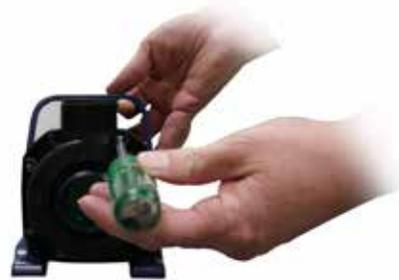
**3** Twist the pump cover to the left to remove the pump cover body.
