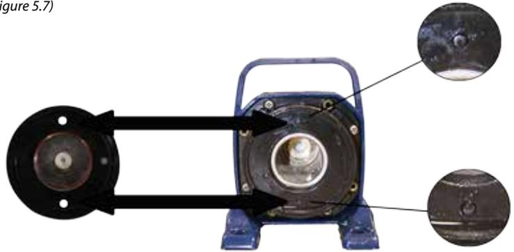
**8** Place the pump body cover 45 degrees to the left and twist to the right to lock into place.
