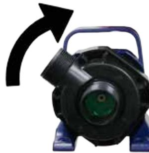
**9** Connect the pump body cover to the pump body and secure by tightening with the 4 screws.
