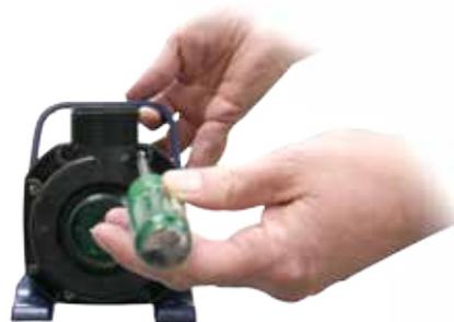
**10** Connect the pre-filter cage to the pump body by sliding into place.
