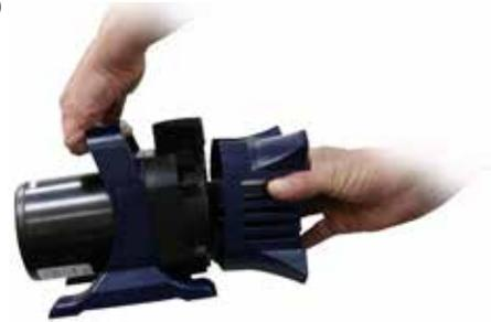
**2** Remove the 4 screws securing the pump body cover to the pump body.
