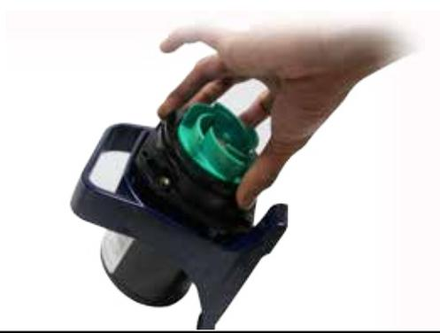
**7** There are pins on the pump body that the impeller will click into. The impeller has openings on the back for the pins to click into.
