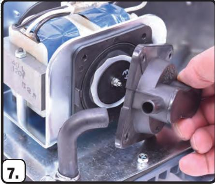
7. Remove diaphragm frame, may need flat head screw driver to separate from unit - note orientation for proper installation of new one (step 8).
