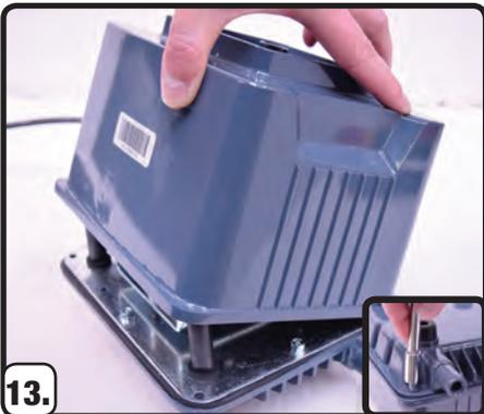
13. Repeat process on other side and reassemble housing, completely dried/cleaned filter and lid.
