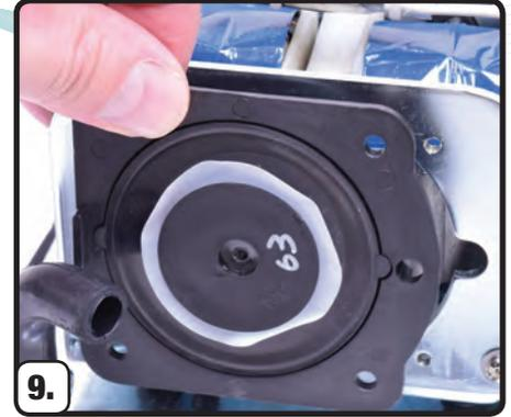
9. Line up new diaphragm to match how old one came off. Match up to notch on motor housing.
