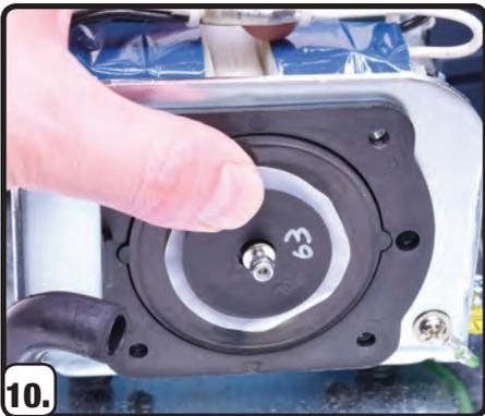
10. Secure diaphragm to magnet with new washer and nut. Push the magnet from behind to help tighten the nut to the magnet. Be sure to get tight. A drop of Blue/Removable Loctite® may be used.
