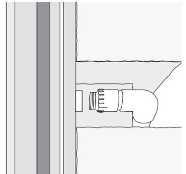
**7** The dual inlet units can be supplied with one mainline. Picture is for illustration only. Application may vary from image shown. After the mainline is split into two, the plumbing lengths to the spillway inlets should be equal. This will ensure equal flow rates to both inlets, while being able to control the overall flow with a single ball valve.
