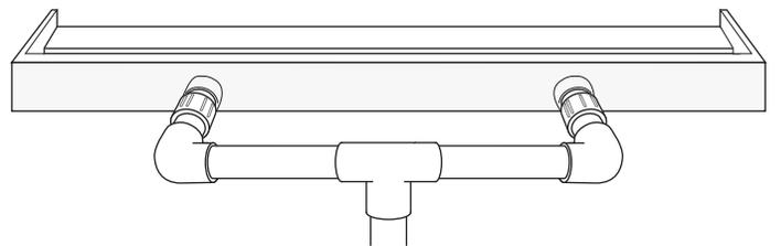
**8** The cord for the LED light strip can be tucked into the notch in the spillway. A dab of silicone should be used to seal the notch on opposing side. Tuck the cord between the blocks to run the cord to the power source. Ideally, run cord through conduit for future maintenance or removal of light strip.
