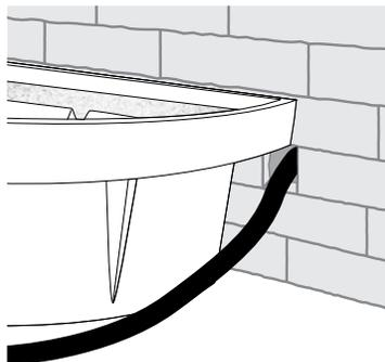
**13** Before gluing black flexible PVC pipe verify the factory installed fittings are tight. Then glue the black flexible PVC pipe into the 45 degree elbow that is pre-installed.
