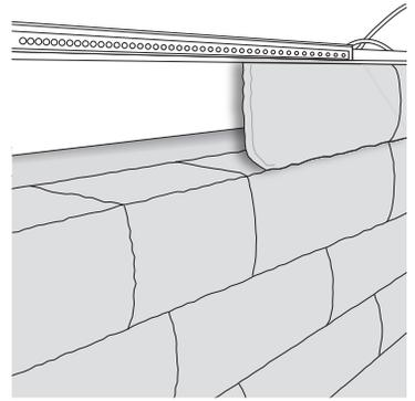
**6** Once the spillway is level and "dry fit" the plumbing can now be fitted. Use the 1" PVC male adaptor and the fittings provided to connect spillway to the flexible PVC pipe. Wrap the threads of the PVC male adaptor with Teflon tape and thread into the spillway inlet(s). Determine the placement of additional fittings (elbows, tees, and extra pipe). Cut and glue all the pieces together to fit the application.
