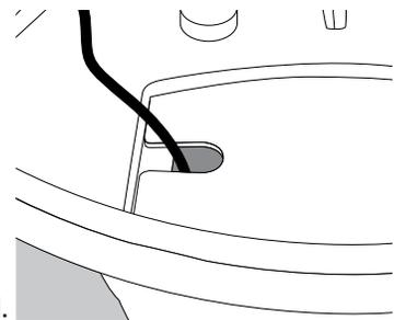
**17** Finish construction of the block wall and any other decorative stone covering the basin. Be sure to leave rock off the area of the splash mat on the basin where the water naturally wants to fall. This will reduce splash and help retain water in the basin.
