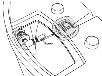
**12** Run the 1" black flexible PVC through the hole previously provided in the block wall. Carefully measure and cut PVC pipe to proper length. Take extra care to verify the spillway has remained in its level position while measuring and cutting the pipe.
