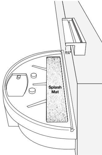
**2** When building the block wall, a section of wall must be left out to accommodate the plumbing and electrical cord for the pump. The notch in the back of the basin is for the power cord of the pump. If an auto fill line is being installed a section of wall should also be open to accommodate the auto fill feed line.
