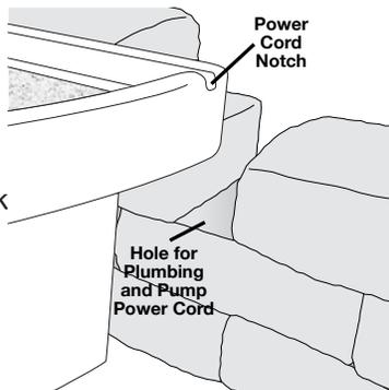
**3** Once the spillway placement has been determined in the block wall, the block will need to be cut to allow for the plumbing connections on the back of the spillway. Use appropriate tools and extreme care when cutting block. Consult block manufacturer recommendations for properly cutting block being used.
