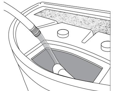
**16** Once proper adjustment of the spillway has been determined, put the pump cover in place. The power cord for the pump can run through the notch in the pump cover. The pump cover can be placed in position as shown or reversed.
