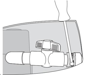
**15** After making sure all plumbing fittings are properly installed, fill the basin with water. The spillway should be tested for proper operation when the wall construction allows. Before final wall installation and covering the basin with rock, the proper flow of the water fall should be adjusted (if needed) with the ball valve on the pump discharge assembly.
