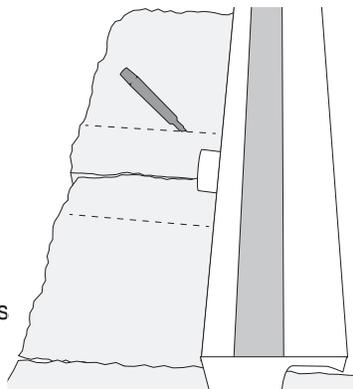
**4** If the lighting option is purchased the LED light strip can be fitted into the back of the spillway. There are brackets on the ends of the light bars with holes in them. These brackets are for other applications. The LED light bar should fit snugly into the back of the spillway. If necessary, a small amount of silicone can be used as an adhesive to hold the bar in place.
